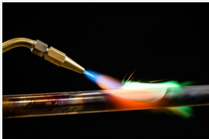
©Bulane – Bulane Oxy-hydrogen flame. An example of a stoichiometric hydrogen-oxygen mixture.
