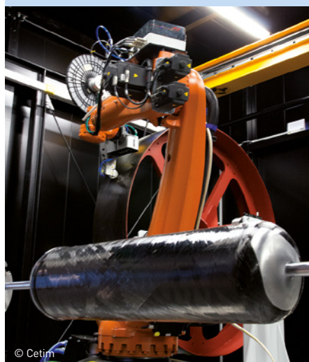
Spide TP, Cetim's new robotised filament winding platform is designed to make large-sized thermoplastic material parts.
